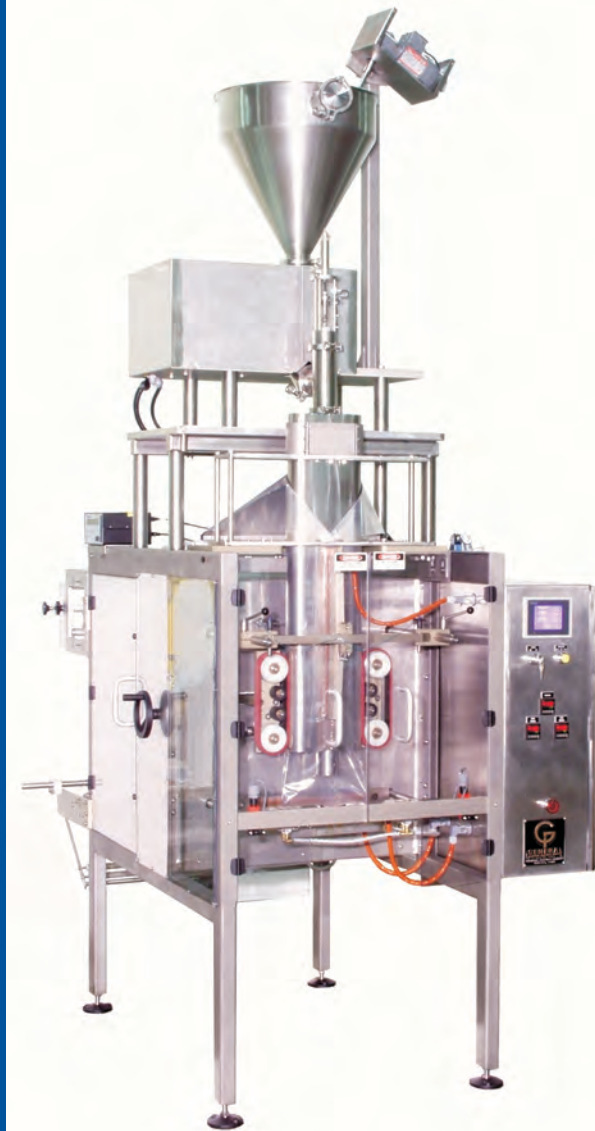
Model 642LP - Stainless Steel Frame Liquid Pump Filler
